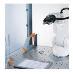
A delicate touch is called for: with great sensitivity, the KR 3 AGILUS fastens micro screws even with a diameter of just 0.8 mm!
